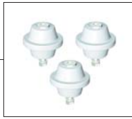
M8 Set of 3 Ø89 x 76 Polyfibre Base Insulators supplied with M7 pedestal base with 3 x 15mm slots on 200mm - 254mm PCD
