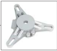
M7 Pedestal Base with 3 x 15mm slots on 200mm - 254mm PCD
